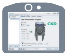
The total mass (Payload) and the position of the center of gravity can be set for tools necessary for robot operation when configuring gripper settings.
