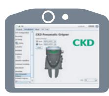
The digital I/O can be configured while viewing a graphic display of the gripper's open/closed status.
