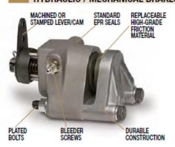
These Tolomatic brakes combine hydraulic and mechanical braking in one caliper. Available in the H/ME20 Series and H/ME20 Series these single acting calipers deliver high braking torque in a small package. Features include: replaceable, high-grade friction material, standard EPR seals, aluminum or cast iron construction (depending on model), bleeder screws and zinc plated bolts. Options include Buna-N seals, Viton® seals and floating brackets. (See pages 50 to 55)
