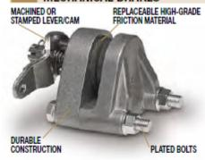
Tolomatic manufactures a broad range of mechanical brakes in these series: ME10, ME20, ME220 and MB3. Designed for use in areas that do not have access to other types of power, these single acting calipers feature replaceable, high-grade friction material, aluminum or cast iron construction (depending on model) and zinc plated bolts. (See pages 56 to 65)
