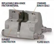
Tolomatic manufactures pneumatic brakes in three sizes: P10 Series, P20 Series and P220 Series. Available in both double acting or single acting. These brakes feature replaceable, high-grade friction material, standard Buna-N seals, aluminum construction and zinc plated bolts. Options include EPR seals, Viton® seals, retractable pistons and floating bracket. (See pages 32 to 37)
